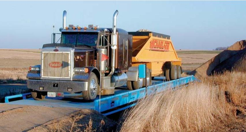
And should the scale need to move, there is no additional expense for building a new foundation. Just pick up the foundation and take it with you.
