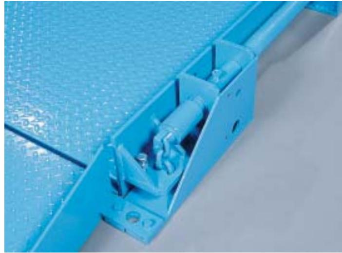
**Suspended deck.** The scale platform is suspended from four Weigh Bars® with simple, trouble free links that require no adjustment. Stops at each corner prevent structural overload and restrict lateral deck movement. The solid steel Weigh Bar weight sensor can take the abuse of tough, industrial usage.
